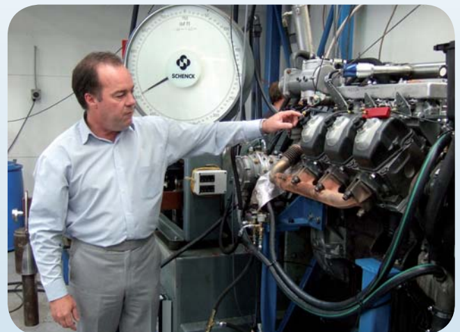
The Actros LPG engine conversion being run through test bed trials
